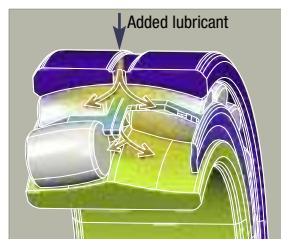
The series 24000 is a very wide series, with extra-long rollers ensuring optimized capacity. Therefore, SNR decided to maintain the lateral shoulders and the central rib.
